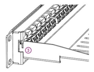
\* For a permanent CMB fixation bend slightly the upper part of the CMB anchor inward using a pointing tool, e.g., a screwdriver.
