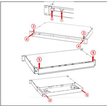
Stage, in its operating position, is fixed by two locating pins **①** affixed to container and anchored in two round openings in stage bottom.
