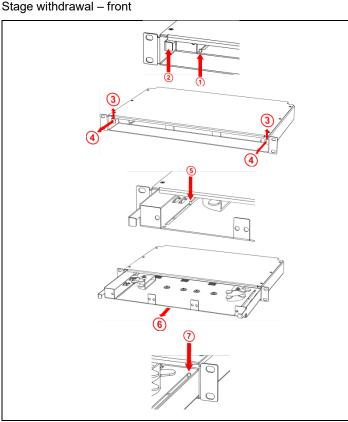
Stage, in its operating position, is fixed by two locating pins • affixed to container and anchored in two round openings in stage bottom.
