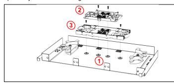
Stage is equipped with four points **①** comprised by embosses with nuts for splice tray/cassette mounting:
