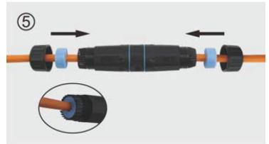
Lock the two waterproof plugs on the cable, then put them into the end of the long tube. Note: The plug is engraved with the word "waterproof" on one side outward.
