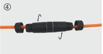
Screw the long tube tightly onto the RJ45 coupler as guided in the manual.
